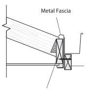
100 x 38 Continuous Ledger fixed to noggings with 2/75 x No. 14 Type 17 Roof Batten Screens at 600 crs. Carport rafters to be fixed to ledger with joist hangers as for Methods F1, F2 & F3.
