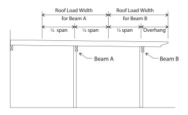
Figure 4 - Roof load width
