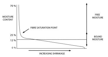
Figure 1. - Shrinkage vs Moisture Content.
