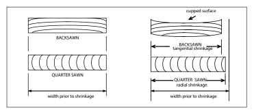
Figure 2. - Relative cupping in backsawn & quarter sawn.
