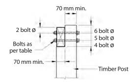
Figure 4 – Example 1 - 1684 typical beam to post detail
