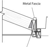
100 x 38 Continuous Ledger fixed to noggings with 2/75 x No. 14 Type 17 Roof Batten Screens at 600 crs. Carport rafters to be fixed to ledger with joist hangers.
