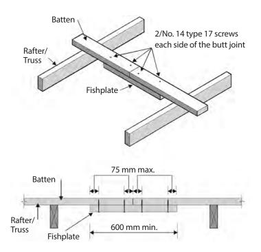
Figure 2 – Joining battens between supports
