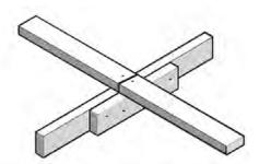
(a) Butt-join with block fixed to side of rafter/truss
